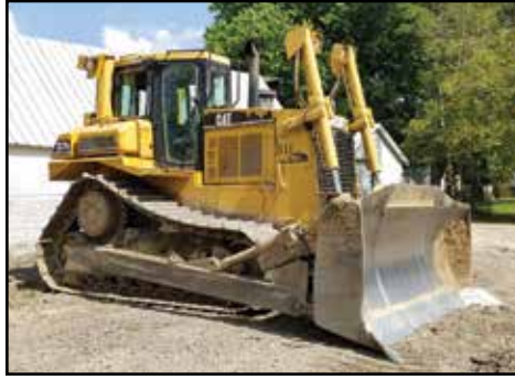
CATERPILLAR D7R Series II Crawler Dozer
